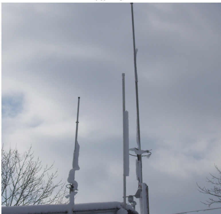
The antenna on the left is a Ringo Ranger 2M; the next is a dual band 2/440 that uses a 6 ft. piece of PVC pipe; the one on the right is a Cushcraft AR-10 Ringo.
